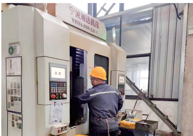
Automated CNC (vertical) deep hole drilling
