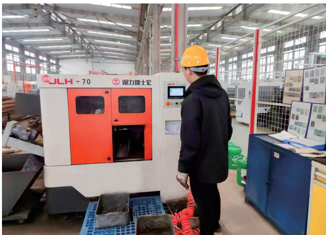
Automated CNC circular saw machine
