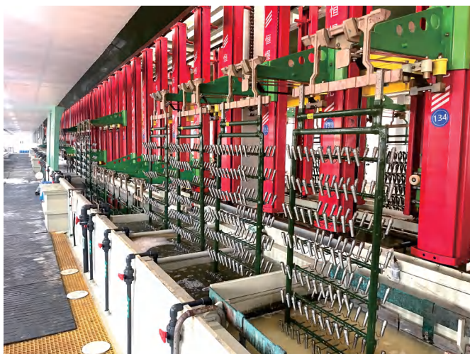
Automated ring-type plating production line
